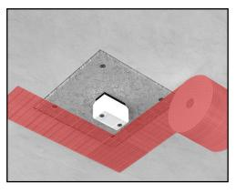
10. Tape the seams between the drywall board and ceiling. Joint compound may be used to fill any gaps before applying the tape.
