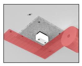
13. Tape the seams between the drywall board and ceiling. Joint compound may be used to fill any gaps before applying the tape.
