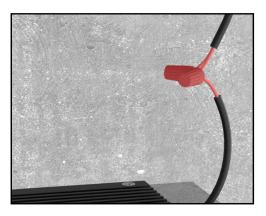
9. Feed low voltage wiring to the bracket and lift the fixture board assembly to the low voltage electrical connection and make the connection.
