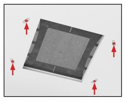
4. Take the drywall bracket and insert it into the ceiling opening. Insert the screws included with the universal drywall bracket through the drilled holes.
