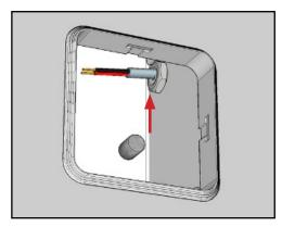
4. Bring low voltage wiring from the remote power supply to the housing and feed low voltage wires through the cable gland opening.
