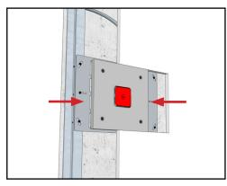
8. Cut and install the drywall around the fixture, ensuring that the fixture board assembly is flush with the surrounding drywall. This will allow a finish of one eight inch of plaster around the finishing guard.
