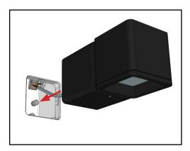
13. Make the low voltage electrical connection.
