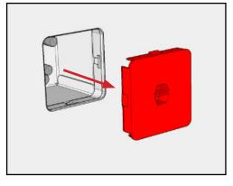
12. Carefully remove the finishing guard from the fixture opening.
